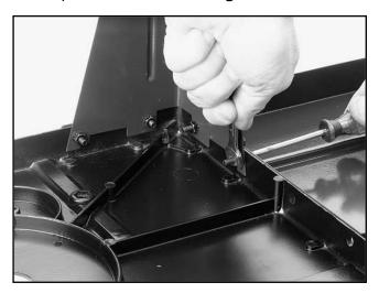
**Figure 5.** Securing a leg to the main table.
